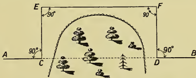
FIG. 78.—Prolonging Chain Line past Obstruction.
